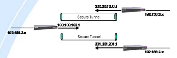
The final type of VPN setup is the **Client to Gateway**. A good example of where this can be applied is when a remote sales person accesses the corporate network over a secure VPN tunnel.
