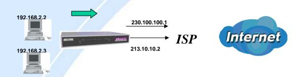
In the above example, PC 1 (IP\_192.168.2.2) and PC 2 (IP\_192.168.2.3) are connected to the Internet via WAN1 (IP\_230.100.100.1) and WAN2 (IP\_213.10.10.2) on BiGuard 30. You can configure BiGuard 30 to balance the load of each WAN port with one of two mechanisms:
