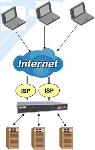
DNS Inbound is a three step process. First, a DNS request is made to the router via a remote PC. BiGuard 30, based on settings specified by the user, will direct the requesting PC to the correct WAN port by replying the selected WAN IP address through the built-in DNS server. The remote PC then accesses the network via the specified WAN port. How BiGuard 30 directs this traffic through the built-in DNS server depends on whether it is configured for Fail Over or Load Balancing.
