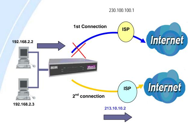
In the above example, PC 1 (IP\_192.168.2.2) and PC 2 (IP\_192.168.2.3) are connected to the Internet via WAN1 (IP\_230.100.100.1) on BiGuard 30. Should WAN1 fail, Outbound Fail Over tells BiGuard 30 to reroute outgoing traffic to WAN2 (IP\_213.10.10.2). Configuring your BiGuard 30 for Outbound Fail Over provides a more reliable connection for your outgoing traffic.
