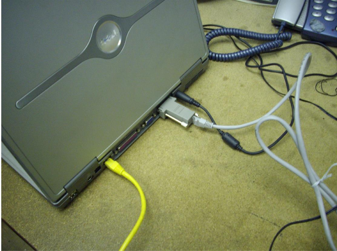
4. Connect up an Ethernet cable (RJ45) from the RS232 to Ethernet converter to the 74xx LAN port 4, then insert a second RJ45 cable into the computer's LAN port and the other end of the RJ45 cable to LAN port 1 on the 74xx.
