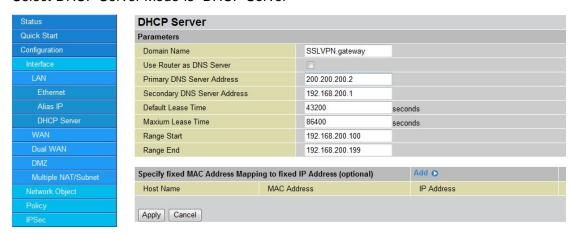
Please uncheck the box"Use Router as DNS Server",set"Primary DNS Server Address" and "Secondary DNS Server Address".Once finish enter the settings then click on the "Apply"button. To save the setting permanently.
