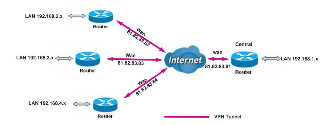
in each spoke router, you configure a VPN tunnel to the hub with a **destination netmask of 255.255.0.0**, indicating that all 192.168.x.x addresses can be reached through the tunnel to the hub. At the hub, we will configure separate tunnels to each spoke with destination netmasks of 255.255.255.0. The tunnels from the hub will have **source netmasks of 255.255.0.0**, indicating that hosts from any 192.168.x.x address can access the tunnel to the spoke.
