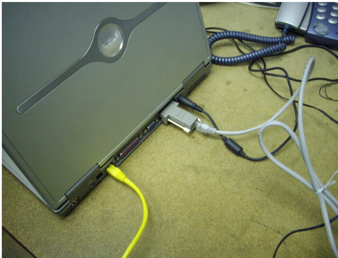
3. Plug the other end of the console cable to your PC's serial port
