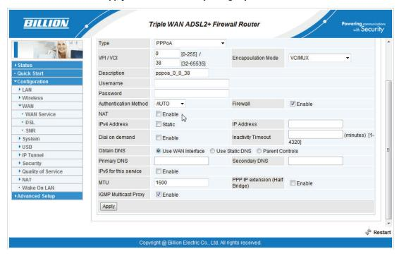
In this mode the 8800NL will present multiple WAN IPs to multiple devices. Each device can have its own public IP address based on your setup and preferences.
